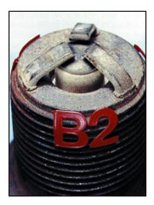
This plug was returned to us as one of a set of 12 that had operated for approximately 4000 hours in the fuel cells (pre-combustion chambers) of a turbocharged, four-stroke cycle, stratified charge, natural gas-fueled, stationary, V-angle, slow speed, 12-cylinder, integral compressor engine.
