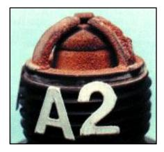
This plug was returned to us as one of a set of 16 that had operated for only 200 hours in a turbocharged, four-stroke cycle, low Btu digester gas fueled, stationary, V-angle, hot water cooled, 16-cylinder engine driving a generator at 1200 rpm.
