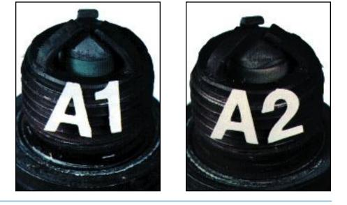
A. R. Brenholts, Jr. is President - Chief Engineer Stitt Spark Plug Company, Conroe, Texas, U.S.A. The plug in Case A is one of a set of 12 that had operated for approximately 2000 hours in a naturally aspirated, four-stroke cycle, natural gas fueled, stationary. V-angle, 12-cylinder engine driving a separable compressor at approximately 1000 rpm.
